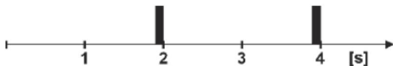
Sensor on standby, no obstacles in the detection area.
